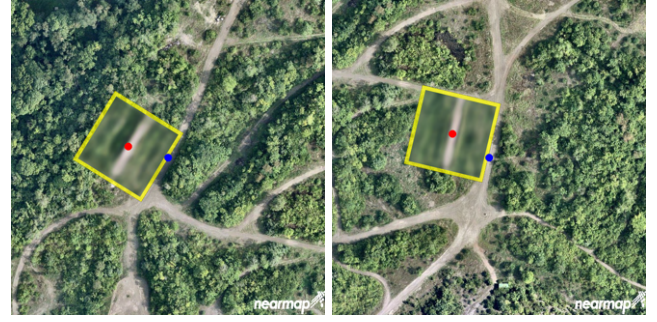
Fig. 6. Examples of failure cases due to the uniform weighting of NCC.
