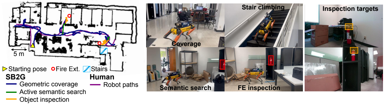
Fig. 5: Experimental results of real-world autonomous inspections using SB2G. The left figure compares the SB2G’s robot paths with paths manually operated by a human during the search and inspection of fire extinguishers. The middle figures show our legged robot performing geometric coverage, semantic search, fire extinguisher inspection, and stair climbing. The right figures provide the camera view of the robot, demonstrating its capability to inspect the gauge of the fire extinguisher.
