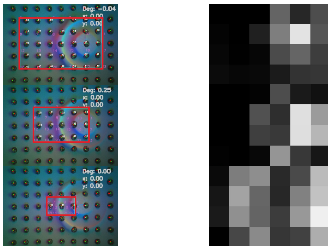
Fig. 7: The user can specify the location and spacing of the sampling grid, in order to resolve higher levels of detail. From top to bottom, the sampling spacing is 45, 30, and 15 pixels.
