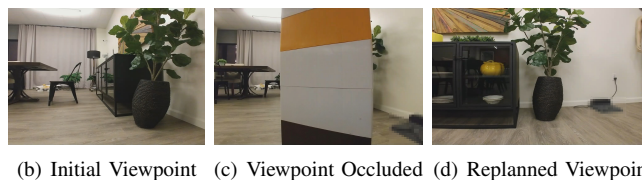
Fig. 1: (Fig. 1-a) The overall framework of VLPG-Nav. Given an object-related prompt, an initial viewpoint is computed using the visual language pose graph (VLPG) and clustering. Subsequently, we center the object in the camera image through our proposed object-centering cost function. If the object is not in view at the chosen viewpoint, we replan using an object localization probability map constructed using the local occupancy map and VLPG. (Fig. 1-b) A real-world example where the robot is tasked with viewing a plant . The figure shows the camera view from the initial viewpoint, and the robot successfully views the plant. (Fig. 1-c) In this case, we obstruct the initial viewpoint with an obstacle. The figure shows the obstructed camera view from the initial viewpoint. (Fig. 1-d) Due to occlusion, the local search identifies an alternative viewpoint, enabling the robot to achieve an unobstructed view of the plant.
