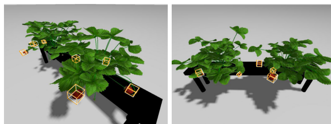
Fig. 4: Inferences made on the synthetic test dataset. The orange 3D bounding boxes represent our predictions of the strawberries, as well as the white ones denote the ground truths.
