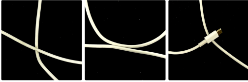
Fig. 7: Three potentially ambiguous configurations for cable tracing. Left: Cable crossing. Center: Tangential contact. Right: Endpoint contact.
