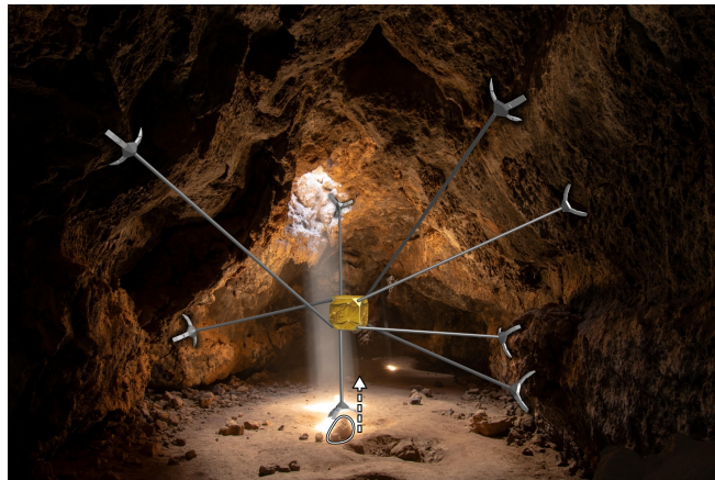
Fig. 1. ReachBot performs a sample-extraction manipulation task in a cave environment. By optimally planning (i) where to place the booms and (ii) the tensions in each boom, we ensure that this task is completed even with uncertain pose and wrench estimation, and stochastic failure modes.
