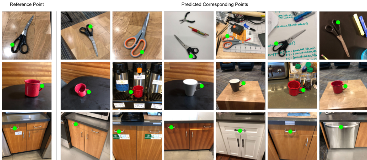
Fig. 5. In Diffusion-PbD, features from a pre-trained Stable Diffusion [52] image model are utilized to transfer demonstrated contact points to new scenes. The examples in this figure show the effectiveness of this method at finding corresponding points in novel viewpoints, objects, and scenes. The reference points on the left are extracted from human demonstrations, and the corresponding points on the right are predicted through the use of diffusion features.
