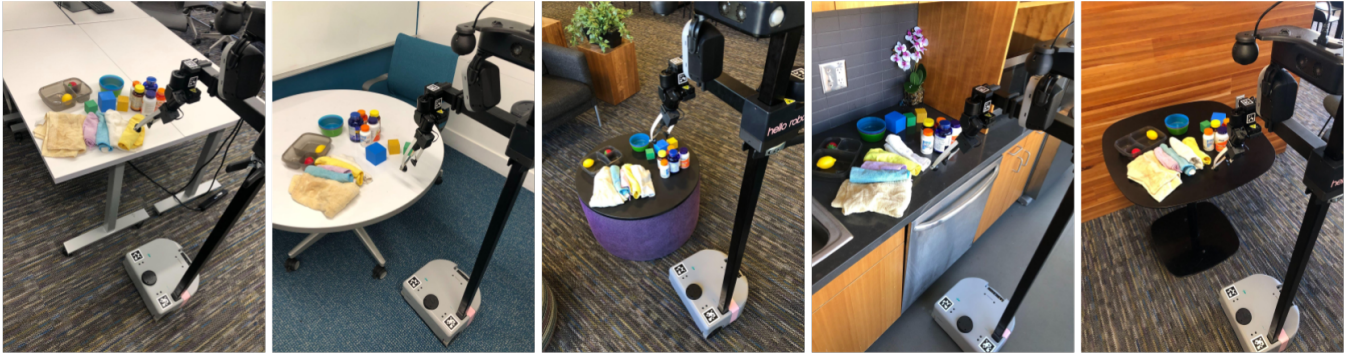
Fig. 6. We evaluate Diffusion-PbD using a Stretch RE2 robot to perform 14 real world manipulation tasks across 5 visually distinct environments. We show that this approach is effective for single-shot imitation of a wide range of manipulation tasks and generalizes to novel viewpoints, objects, and scenes.
