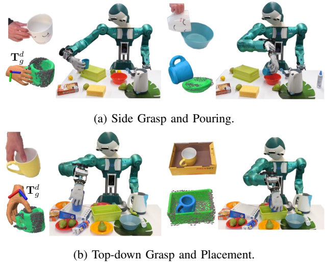
Fig. 1: Learning task-oriented object grasping and rearrangement from human demonstration videos of manipulation tasks. We illustrate two tasks: (a) side picking a mug and pouring into a bowl; and (b) top-down picking a mug and placing it into a container. For each task, we show the RGB image, the observed point clouds ( \bullet ), reconstructed object meshes ( \blacksquare \blacksquare ), extracted hand mesh ( \blacksquare ), grasp poses ( T_g^d ), and the execution on a humanoid robot.
