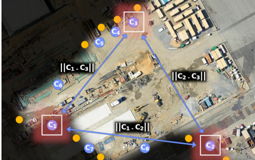
Fig. 4: Heuristic to pick new rendezvous locations when robots have common information during synchronization for 3 sub-teams from the example from Fig. 3 in a construction site. The orange circles are frontiers, and the blue circles are the center of masses obtained from the KNN algorithm. The center of masses c_1 and c_3 were chosen to the 1 st and 2 nd sub-teams. Differently, c_2 was chosen to the 3 rd sub-team by maximizing the distance \sqrt{(c_1 - c_2)^2 + (c_2 - c_3)^2} .
