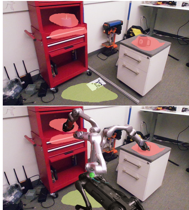
Fig. 1: Spatial Diagrammatic Instructions enable users to sketch on camera images of the environment. Top: Red indicates regions where the user sketches as regions of interest, while green indicates regions the user sketches as permissible regions. Bottom: Continuous spatial representations of these sketched regions can then be incorporated as objectives and constraints within optimization problems to find optimal positions for mobile manipulator base placement.
