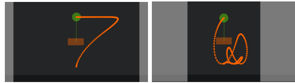
Fig. 6. The trajectories \mathbf{x}_0^* , \mathbf{x}_K^* found by P-HO shown from left to right. As we go from \theta_0 to \theta_K , m_{pole} increases from 1kg to 60kg and F_{max} goes from 200N to 100N thus more swings are needed.
