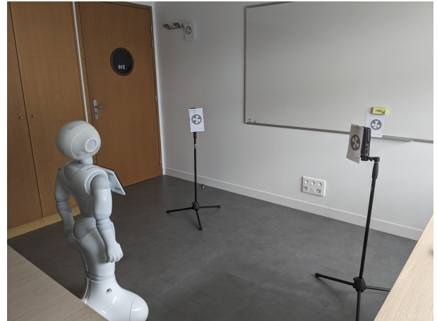
Fig. 6. Landmarks recognized by Pepper were set up in the room to mimic objects. The human stood in front of the robot.
