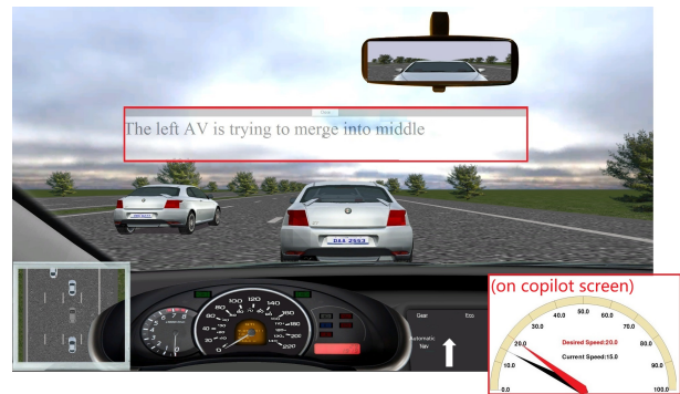
Fig. 3: The simulated windshield projection system (middle) and the visual display of the current speed and the desired speed (bottom right).
