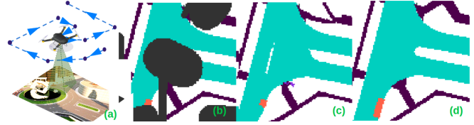
Fig. 1. (a) Semantic coverage mapping is performed by a UAV in an urban environment using a downward-facing sensor with a limited field of view. (b) Only a partially revealed map can be obtained if time or energy is tightly constrained (dark color represents missing regions. See Fig. 6 for other colors). (c) Our proposed SePaint is able to reason about the underlying semantic structures. (d) Ground truth of the environment.
