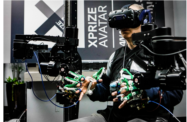
Fig. 1: SNU-Avatar haptic glove is installed on the haptic device and is being operated by an operator.
