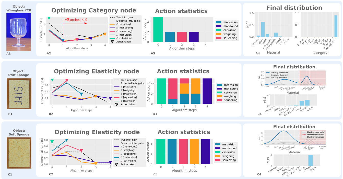
Fig. 5: System operation and performance – examples. (Left – A1/B1/C1) Object name and image. (A2/B2/C2) Single run of experiment with termination criterion off. Expected IG of the actions shown. Triangle markers show which action was chosen in a given step. The dashed black line shows the experimental true IG after the action was executed. This action is not shown anymore in subsequent algorithm steps. (A3/B3/C3) Count of actions chosen during the runs with the termination on (if all available actions at a given step had negative expected IG, execution stopped). (A4/B4/C4) Final probability distributions of relevant variables of the single run shown in (A2/B2/C2).
