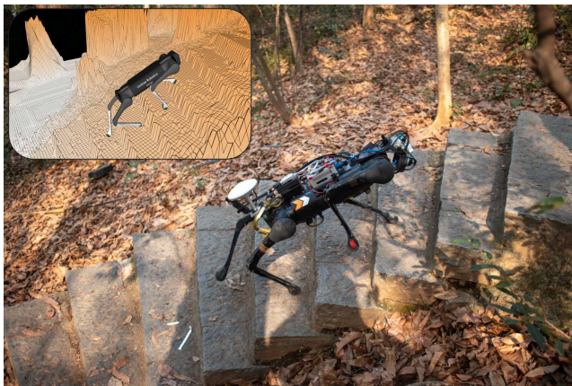
Fig. 1. Aliengo travels outdoors, with the robot autonomously selecting safe and reliable contact positions. The terrain consists of steps of varying widths and heights. Uneven surfaces and irregular steps pose a challenge for Aliengo.
