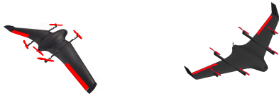
Fig. 8. (Left) PX4’s Deltaquad QuadPlane VTOL model. (Right) The modified model has six vertical rotors and disables the horizontal rotor.
