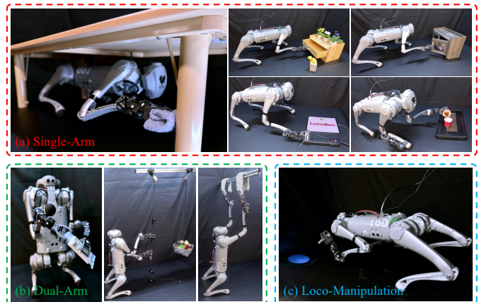
Figure 1: Equipped with loco-manipulators, LocoMan is proficient in handling versatile manipulation tasks. (a) With a single loco-manipulator, LocoMan not only can perform manipulation tasks that require precision and stability, but also excels at operating in extremely narrow space in its compact form. (b) With both loco-manipulators installed on the two front legs, LocoMan is able to perform bimanual manipulation tasks when standing upright. (c) LocoMan is also capable of loco-manipulation, e.g. carrying objects with its loco-manipulators while walking.
