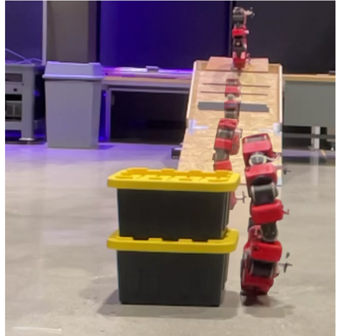
Fig. 1. Illustrates a frontal view of COBRA [11]–[13] engaged in tumbling while navigating around an obstacle using posture manipulation.
