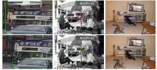
Fig. 9: Deep visualization of qualitative comparison between previous best model Top : AirDet (baseline) and Bottom : Airshot (ours). AirShot can focus more precisely on the most representative part of the object, resulting in more accurate box regression.
