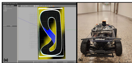
Fig. 3. (a) The simulator and (b) robot vehicle used as a sim-to-real validation pipeline for the ROBOCOP framework.
