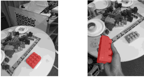
Fig. 2: Example illustrating the benefit of user-object interactions for object discovery. Toy bricks of different sizes are placed next to each other in a 4 by 3 grid, out of which a 4 by 1 brick is picked up. Left: The closest mask found by a state-of-the-art segmentation network [9] in the static scene in terms of intersection over union with the actual 4 by 1 brick’s mask. Right: Object mask discovered by leveraging the handheld interaction, using our method.
