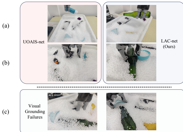
Fig. 6. Examples of the robotic grasping between the baseline method and our method in multiple-object scenes. (a) Successful grasps. (b) Failed grasps. (c) Instances of visual grounding failures.
