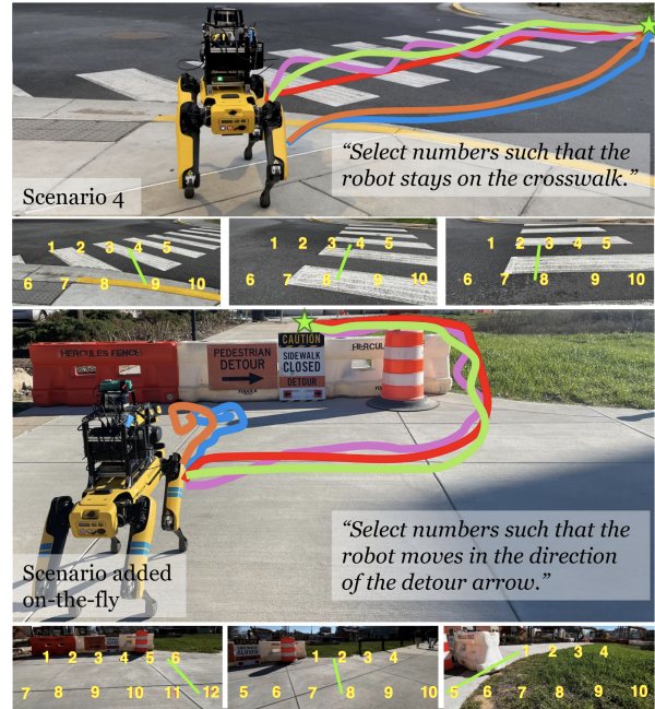
Fig. 1: [Top]: The trajectories of a Spot robot crossing the road when using CoNVOI with GPT-4v [1] (in green), CoNVOI with Gemini [2] (in purple), teleoperated by a human (in red), GA-Nav [3], and DWA [4]. CoNVOI navigates the robot on the crosswalk by understanding the environmental context. [Bottom]: The trajectories when the Spot robot navigates to a goal beyond a blockade. While using CoNVOI, handling such scenarios can be added on the fly using a simple text prompt without any reformulation. The RGB images from the robot are shown with CoNVOI’s multi-modal visual marking (numbers in yellow). GPT-4v/Gemini is queried with the marked image and a context-based text prompt in quotes, and it returns the green reference path that follows explicit, and implicit social rules, and human-like preferences during indoor and outdoor navigation.
