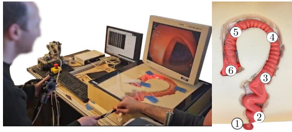
Fig. 5: (Right) Picture taken while collecting data from the expert user. (Left) The silicon model of a colon with numbered landmarks indicating the different segments of the intestine: ① starting location; ② rectum→sigmoid colon; ③ sigmoid→descending colon; ④ descending→transverse colon; ⑤ transverse→ascending colon ; ⑥ ascending colon→cecum.
