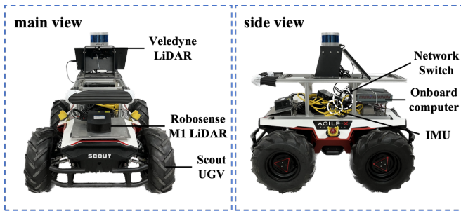
Fig. 4. Our experimental platform, Scout 2.0 is a four-wheeled differential mobile robot equipped with WT-GAHRs1 IMU, RS-LIDAR-M1, and Velodyne VLP-16 LiDAR. The onboard computer used for executing computational processes features an i5-9400H CPU and a GTX-1650 GPU. The sensor configuration in both the simulated and real environments is consistent. The VLP-16 LiDAR is mounted at the center of the UGV, 0.8 meters from the ground, while the RS-LiDAR-M1 is positioned at the front of the UGV, angled downward by 15 degrees.
