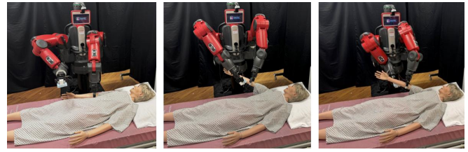
Fig. 6. Snapshots for bimanual bed bathing manipulation task execution in real world. Our experiment includes a bimanual Baxter Humanoid robot, a medical manikin, a hospital bed, and a cleaning tool. In real world, we only evaluate for forearm and upperarm due to the limitation of Baxter’s payload. Example trials can be found in the supplementary video.
