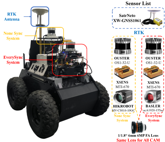
Fig. 7. The real-world experiment platform: A mobile robot base carries both Sync and Non-Sync multi-sensor system.
