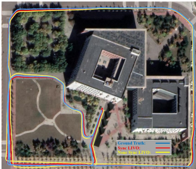
Fig. 8. The RTK ground truth and LIVO trajectories from different sensor suite are plotted on Google Maps.
