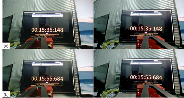
Fig. 6. Precision Experiment for multi-cams. (a) Image pair captured by different cameras at the same time. (b) A later image pair.
