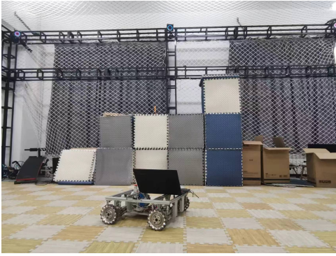
Fig. 4: Experiment overview. The field is 6 \times 8 m, with 8 cameras on top of the field capturing the pose and position of the robot. A target for the capturing system is fixed on the side of the robot.
