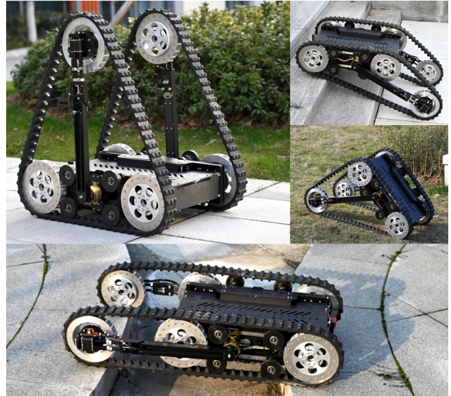
Fig. 1: Prototype of CubeTrack robot with different configurations, including configurations for climbing stairs, lifting chassis, and crossing gaps. Long flippers provide the robots with good obstacle-crossing capability by allowing the robot to adjust its configuration to a large extent.
