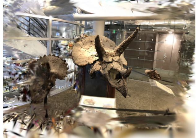
Fig. 1. Our proposed approach enables fast, Gaussian Splatting based 3D reconstruction and photo-realistic novel-view synthesis while simultaneously estimating and refining the camera poses, as visualized on this reconstruction of the horns scene from LLFF [10]. This reconstruction was performed without camera pose information.
