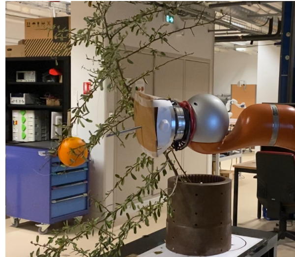
Fig. 1: The robot arm pushes an occluding branch to improve the view of an orange.
