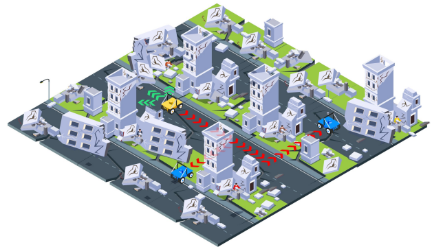
Fig. 1: Search-and-rescue robots collaborate to navigate uncharted disaster zones under realistic communication constraints. For example, the yellow robot must balance trade-offs between disconnecting from its team (blue robots) to independently explore (green arrows), and pursuing other robots to exchange information (red arrows).
