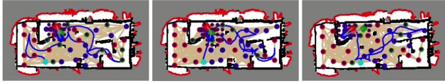
Fig. 8: Snapshot of the final merged graph representations towards the end of an exploration mission for robots 1 (red), 2 (green), and 3 (blue), from left to right. The colored circles represent each of the robot's graph nodes merged from other robots, the colored diamonds their belief positions, and blue trajectories their paths taken.
