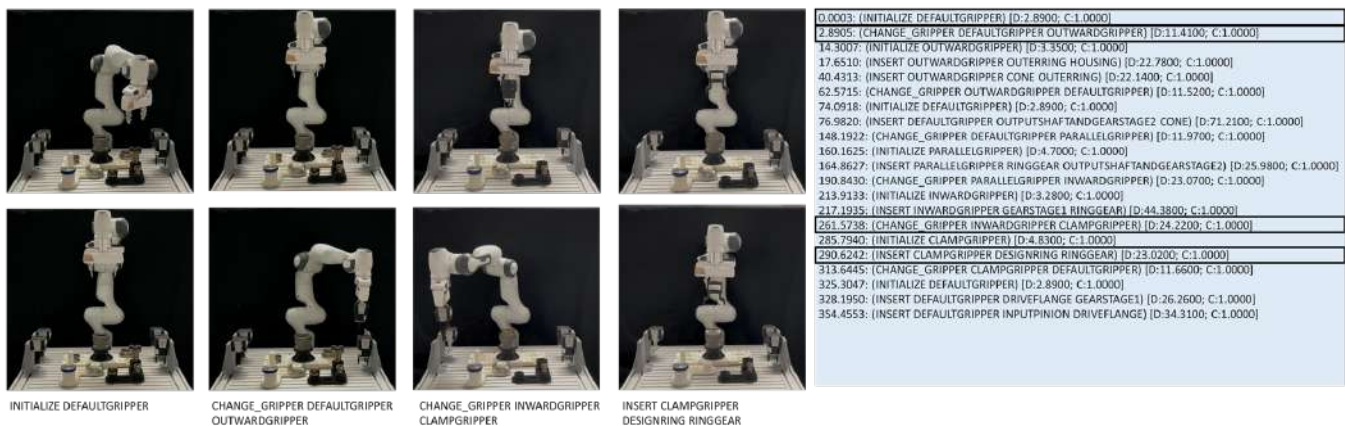
Fig. 5. The planning result and execution of gear assembly in UC 1: picture in each column showcases the pre, executing and post robot state for each planned process
