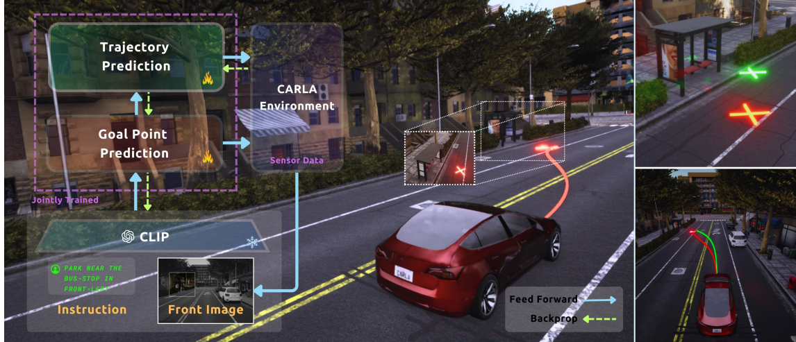
Fig. 1: The proposed method, LeGo-Drive estimates a goal location queried with a navigation instruction- “Park near the bus stop on the front-left” on a single front-facing camera image and coupled it with a differentiable optimizer-based planner that jointly optimizes the trajectory and the goal location. (Left) The proposed architecture is shown along with the gradient flow for joint end-to-end training. (Right-Top) Goal improvement from initial estimation in Green to improved location in Red. (Right-Bottom) Trajectory output in Red leading to the improved goal location, compared with the trajectory generated by baseline in Green.
