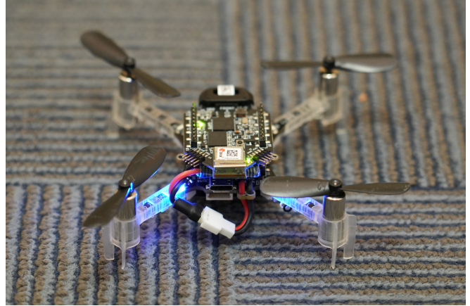
Fig. 1: The Bitcraze Crazyflie 2.1 facing away from the camera with the AI Deck and Flow Deck v2 attached.
