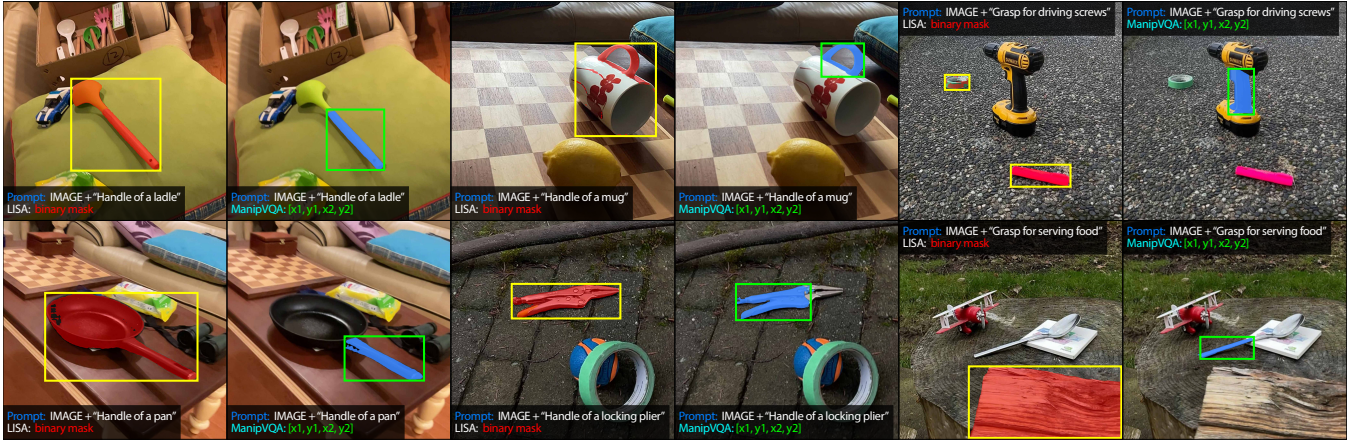
Fig. 3: Illustration of the affordance detection and grounding tasks using the HANDAL Dataset. The first four columns show the results for affordance detection, and the last two columns present the results for the affordance grounding task. In the affordance grounding task, a description of the tool’s intended use is given instead of explicit part names. Blue masks are produced by SAM-HQ based on ManipVQA’s predicted bounding boxes, and red masks are LISA’s output.
