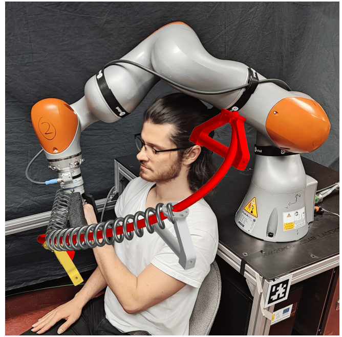
Fig. 6. The virtual mechanism pulls the user perpendicularly towards the curve (yellow) and tangentially to the target (gray). In rotation space, it corrects the orientation to that of the closest point (yellow).
