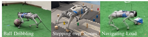
Fig. 1: The proposed HiLMA-Res framework enables a quadrupedal robot to perform different loco-manipulation tasks in the real world. These include dribbling a ball in a desired direction, stepping over small blocks scattered on the ground, and navigating a load to the desired goal through real-world learning. We highlight the versatility of the HiLMA-Res framework in various loco-manipulation tasks with different observation spaces and learning algorithms. We encourage readers to view the supplementary video at https://youtu.be/8dOs9_RDn4E for more results.
