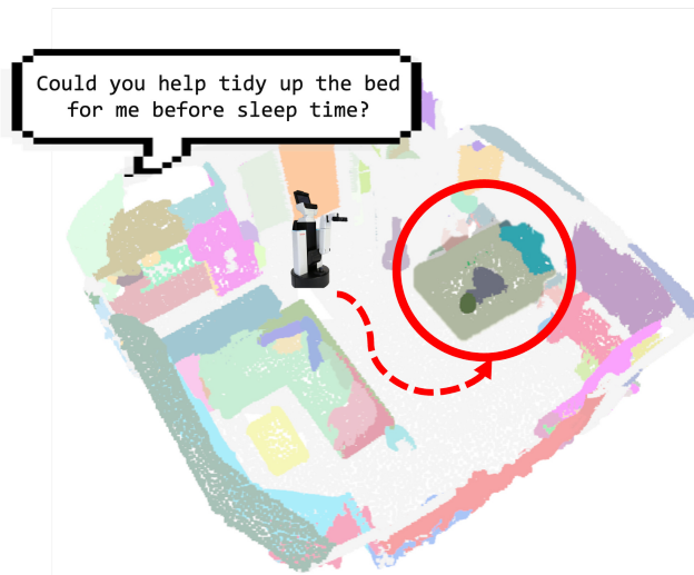
Fig. 1. Illustration of Proposed System. A mobile robot equipped with OV-MAP accurately identifies objects on a per-instance according to input queries.
