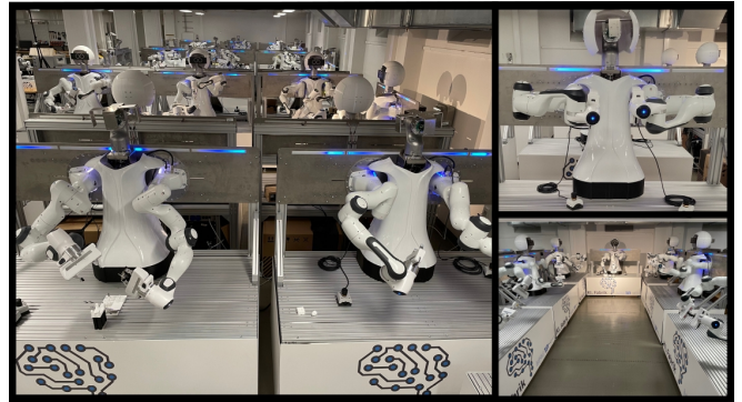
Fig. 2. Picture of the RLUs connected in the PD.RAI platform. Each RLU is a dualarm robot consisting of two Franka Emika Robot arms.
