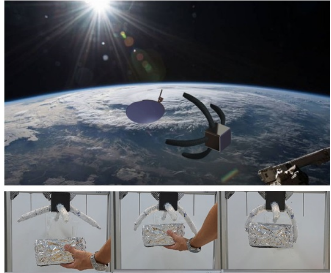
Fig. 1. Thermally-resilient soft manipulator proof of concept designed for active space debris removal missions in Low Earth Orbit (LEO).
