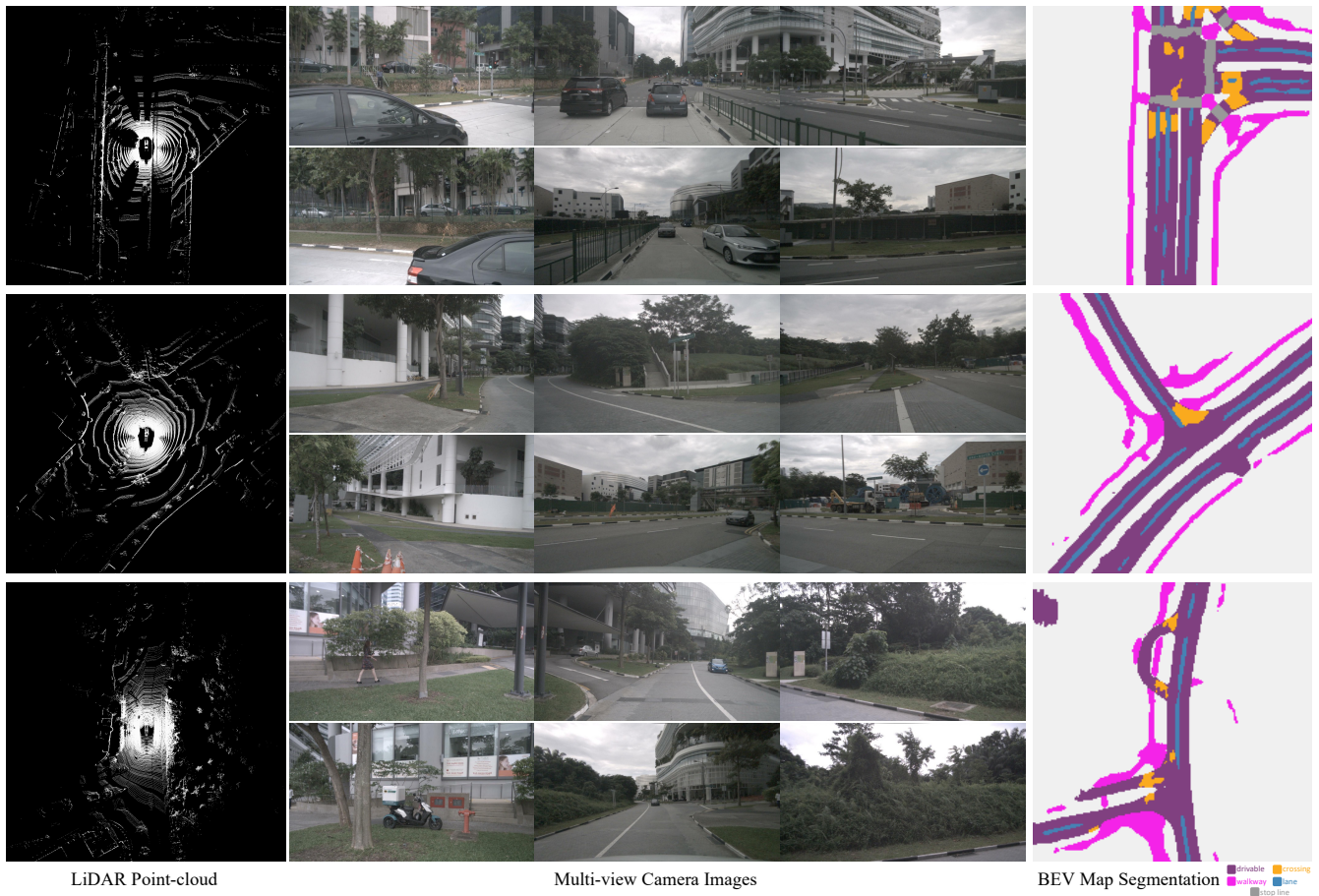
Fig. 3. Qualitative Results. This figure presents the predicted BEV map segmentations across scenes with diverse levels of complexity. The leftmost column illustrates the lidar point-clouds. The middle columns display the six surrounding cameras, arranged from left to right as follows: front-left, front, front-right, back-left, back, and back-right. The rightmost column features the predicted BEV segmentations, with class labels including car park, walkway, lane divider, drivable area, stop line, and pedestrian crossing. The ego-vehicle is positioned at the centre of each map, facing upwards.
