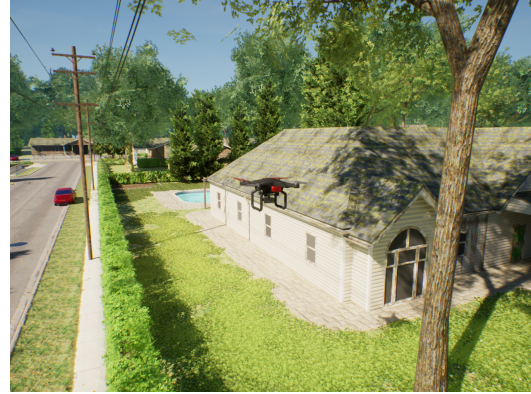
Fig. 1: The neighborhood environment for drone path planning simulated with AirGen, a drone simulator. The other simulated environments for evaluating the algorithms are based on grassland and industrial domains.
