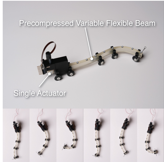
Fig. 1: Top: a 3D printed snake-like soft-bodied robot with a pre-compressed tendon-driven variable thickness flexible beam body. The robot uses only one actuator (a DC motor) to generate traveling mechanical waves along the body to support undulation locomotions. Bottom: snapshots of an undulation motion.
