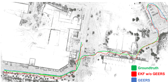
Fig. 8: Long distance experiment using the NCLT dataset. EKF without corrections and groundtruth also shown.
