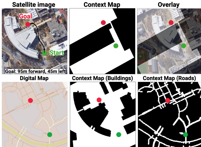
Fig. 2: Top Row: Using a satellite image of the area from Google Maps (left), a human operator sketches a rough Context-Map for the robot (middle). Notice how defective the map is (right): large parts or entire buildings are missing, no roads or sidewalks are shown; but crucially, the map contains a hint for an opening to get to the goal. Bottom Row: Starting from the digital map (left), we automatically generate Context-Maps by segmenting out buildings (middle), or roads (right).
