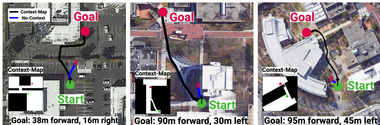
Fig. 5: We test our policies in 3 novel environments in the real-world. The routes contain many obstacles including bushes and buildings, that the robot has never seen during training. The Context-Map policies (black) are able to navigate hundreds of meters to reach the goal 100% of the time. In comparison, the No-Context policies (blue) beeline towards the goal and get stuck on obstacles, resulting in failures.
