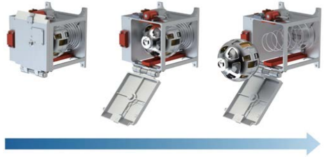
Fig. 11. Stowage box mounted on the ispace Mission 1 lander. The ball-shaped rover is pushed outward onto the lunar surface by a mechanical spring. This box contains a wireless device to communicate to the rover and a data storage to save received images and logs. The size of this box is approximately 120 \times 110 \times 120 mm, and the total mass including the rover and the MLI blankets is approximately 835 g.
