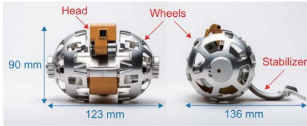
Fig. 2. Deployable components on the rover. The head and the tail stabilizer are deployed after the wheels extend.
