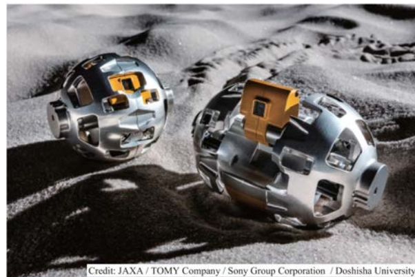
Fig. 1. Picture of the transformable nano rover. The ball-shaped rover on the left side transforms to the wheeled rover on the right side.
