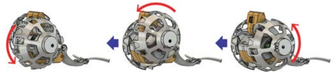
Fig. 7. Motion sequence of the eccentric wheel. This eccentric rotation allows the rover to sweep the wheels with a longer stroke.
